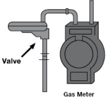
To turn gas off, give the valve a quarter turn in either direction. When the lever crosses the direction of the pipe (see below) the gas is off.
